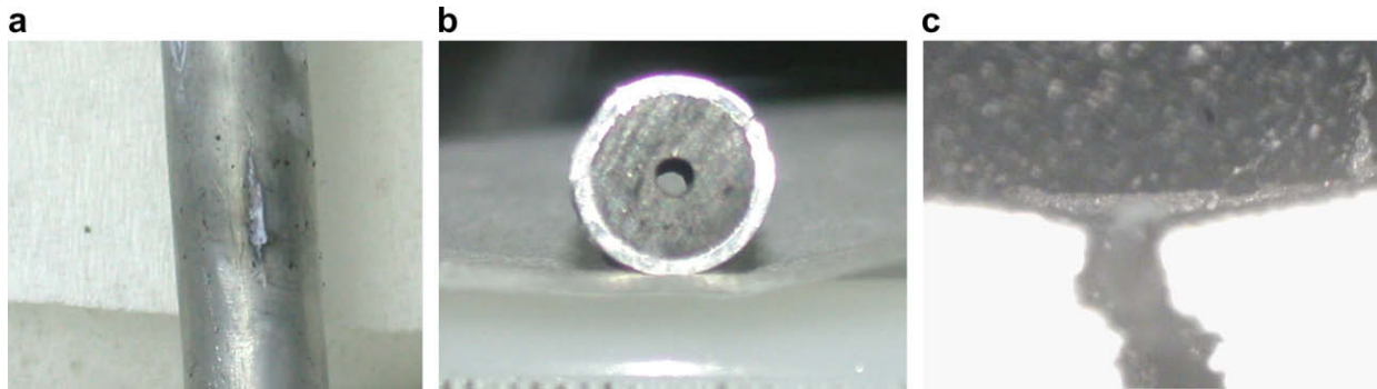
Fig. 2. Photograph of MOX fuel pellets in D9 cladding tube after 350 h at 700 °C; (a) D9 pin showing 'Na' entry through the artificially created breach; (b) cross section of the D9 Pin with annular MOX pellet; (c) breach in D9 cladding and the MOX pellet.
