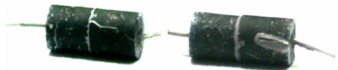
Fig. 5. MOX pellets at 700 °C after 400 h. Showing cracks and sodium patches on the surfaces of pellet.
